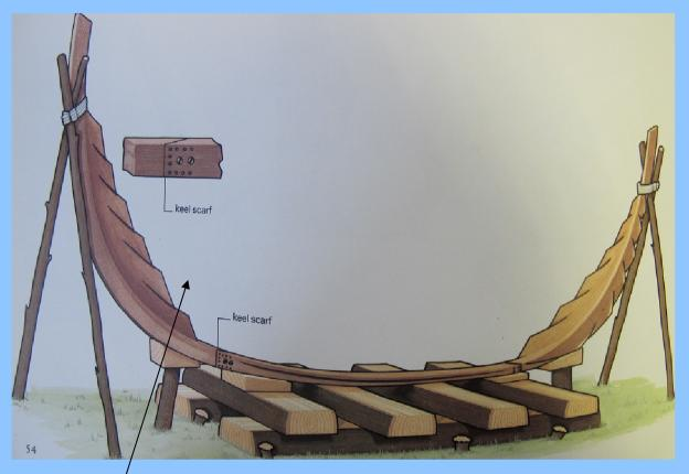
The keel is the backbone of the ship:
