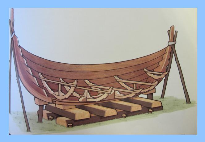
The sides are made of timbers that overlap slightly.
